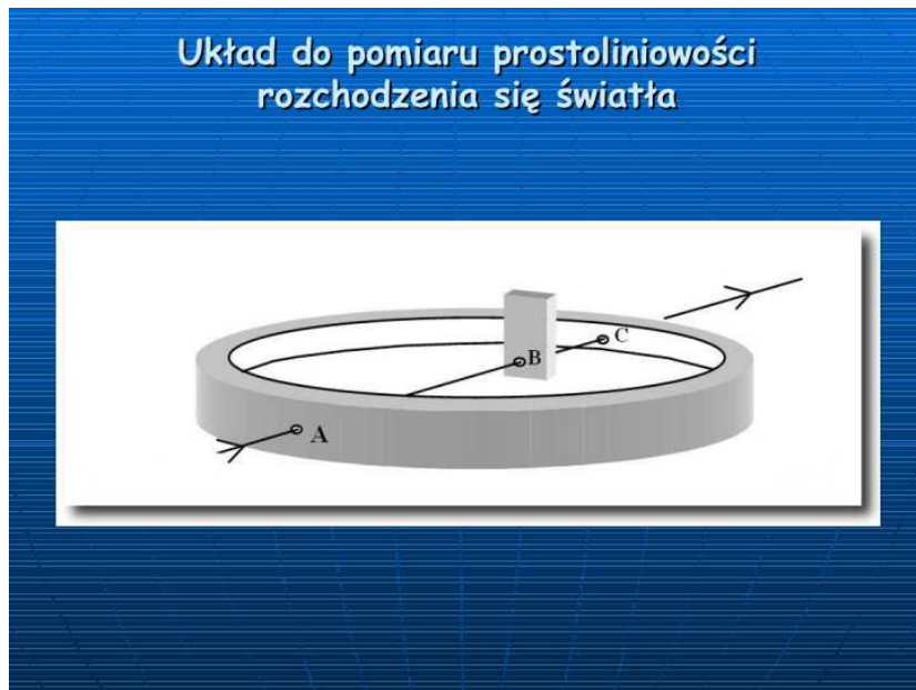
Fig.5. The slide with the scheme of the device for measuring the rectilinear propagation of light
